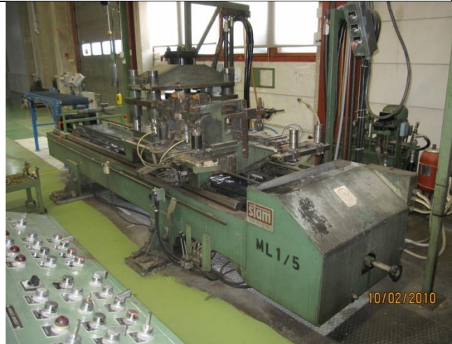
Flying cross cutter, carriage travel speed max. 30m/min (Stam)
