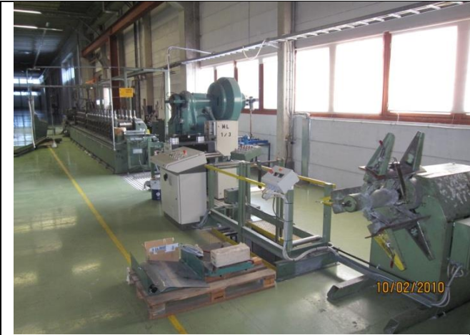
Decoiler 2tn, strip width max. 300 mm (Stam)
