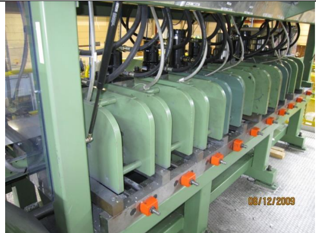
Hydraulic punching unit (P.Oinonen)
