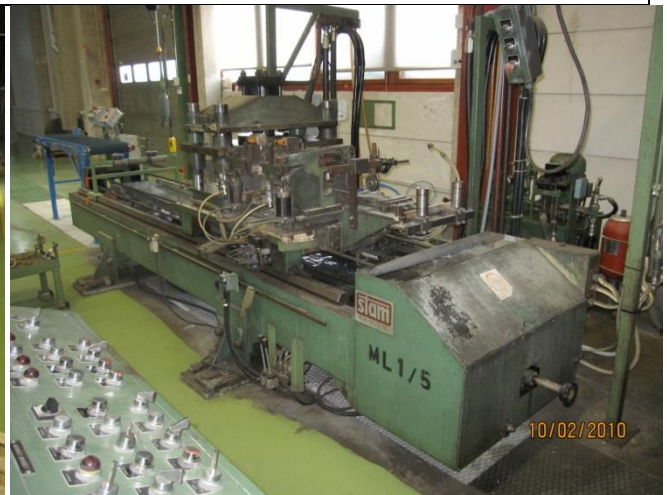
Roller feed unit (Camu) Eccentric press 60 tn (BMP)
