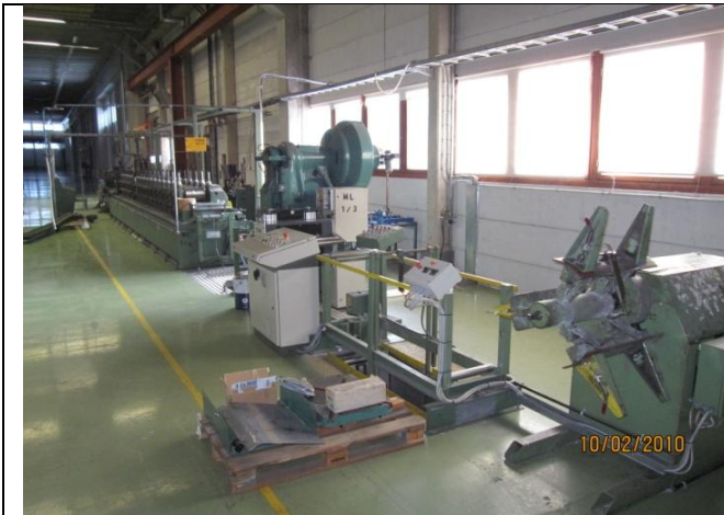
Decoiler 2tn, strip width max. 300 mm (Stam)
