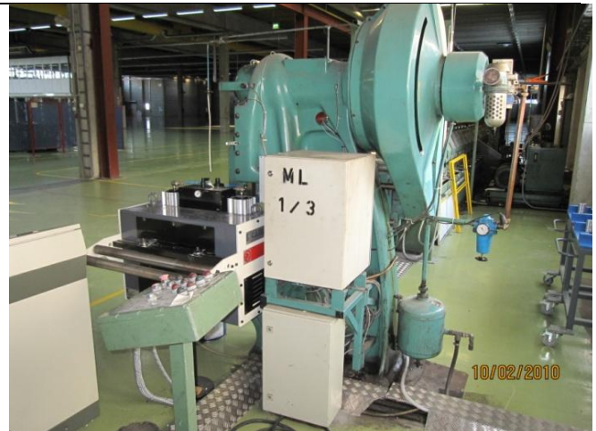
Roller feed unit (Camu) Eccentric press 60 tn (BMP)
