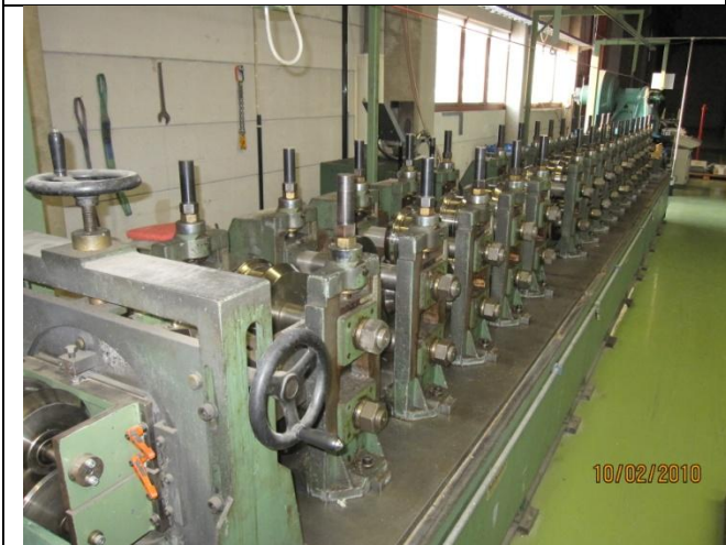
Roll forming machine, 16 stands, strip width 300 mm (Stam)
