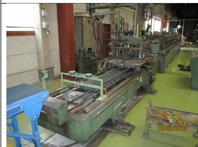
Roll forming machine, 16 stands, strip width 300 mm (Stam)
