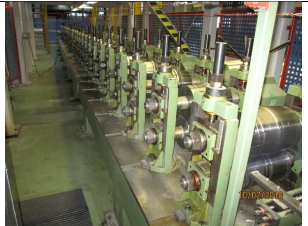
Roll forming machine, 27 stands, strip width 400 mm (Stam)
