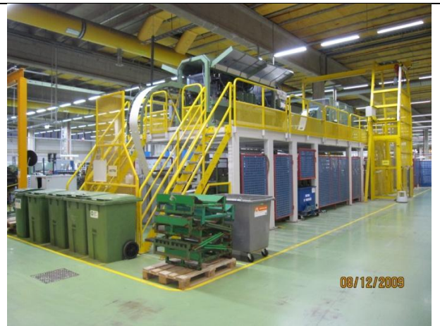
The roll forming line has been used for manufacturing of body plates for light fittings.
